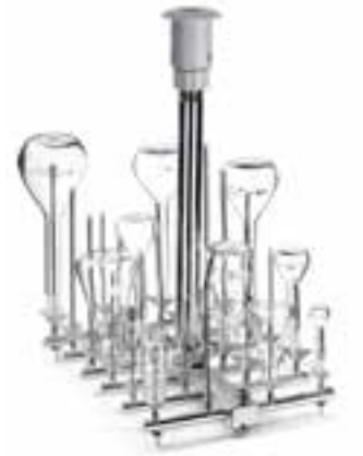
LM24 (only for GW2145 model) Universal 24-position stainless steel flask washer, suitable for washing narrow-necked glassware up to 490 mm in height. Fitted with the following nozzles: 6 x U6240, 5 x U6220, 6 x U4160, 5 x U4140, 2 x U3110. Positioning on the D-CS2 rack lower level.
